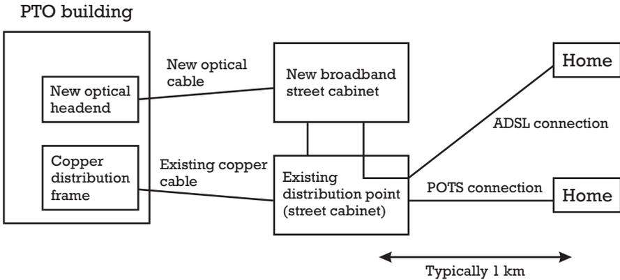
**Figure 3.2** Modifications required to install xDSL technologies.
