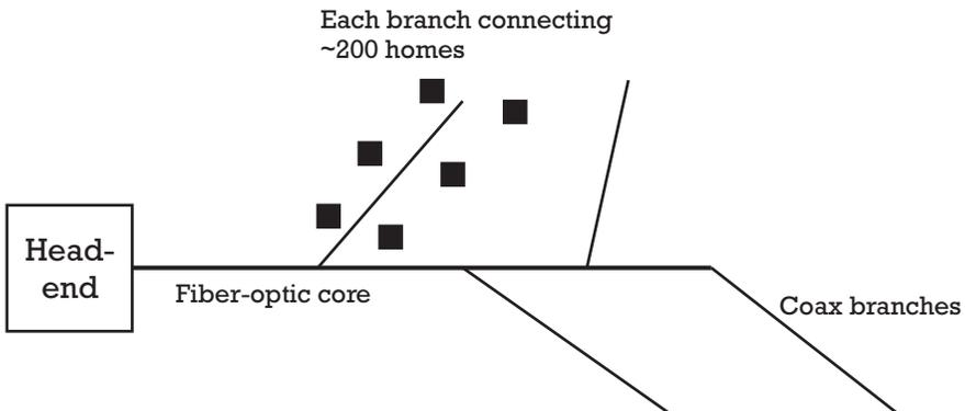
**Figure 3.4** Tree-and-branch architecture.
