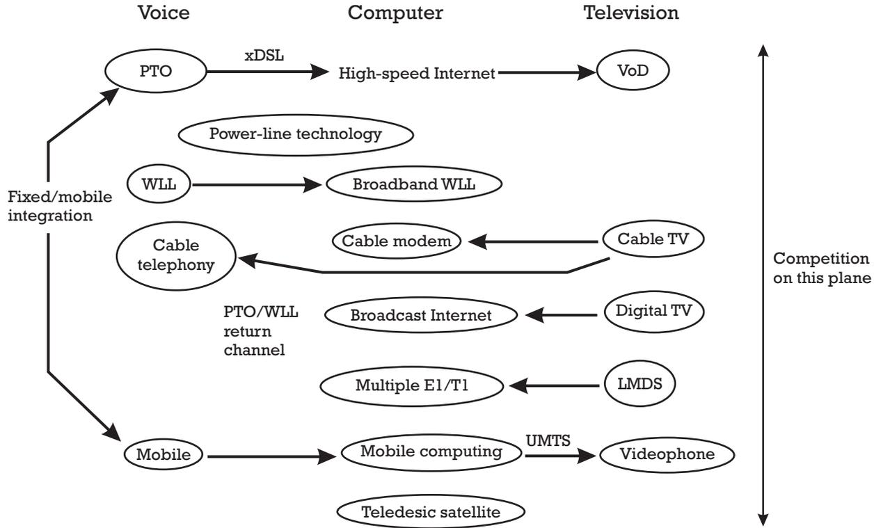
Figure 3.1 Overview of different access technologies.
